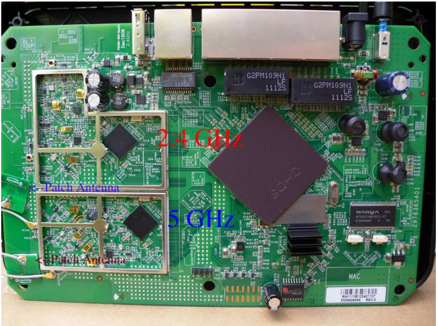
Inside of the Netgear WNDR3700 v.2
