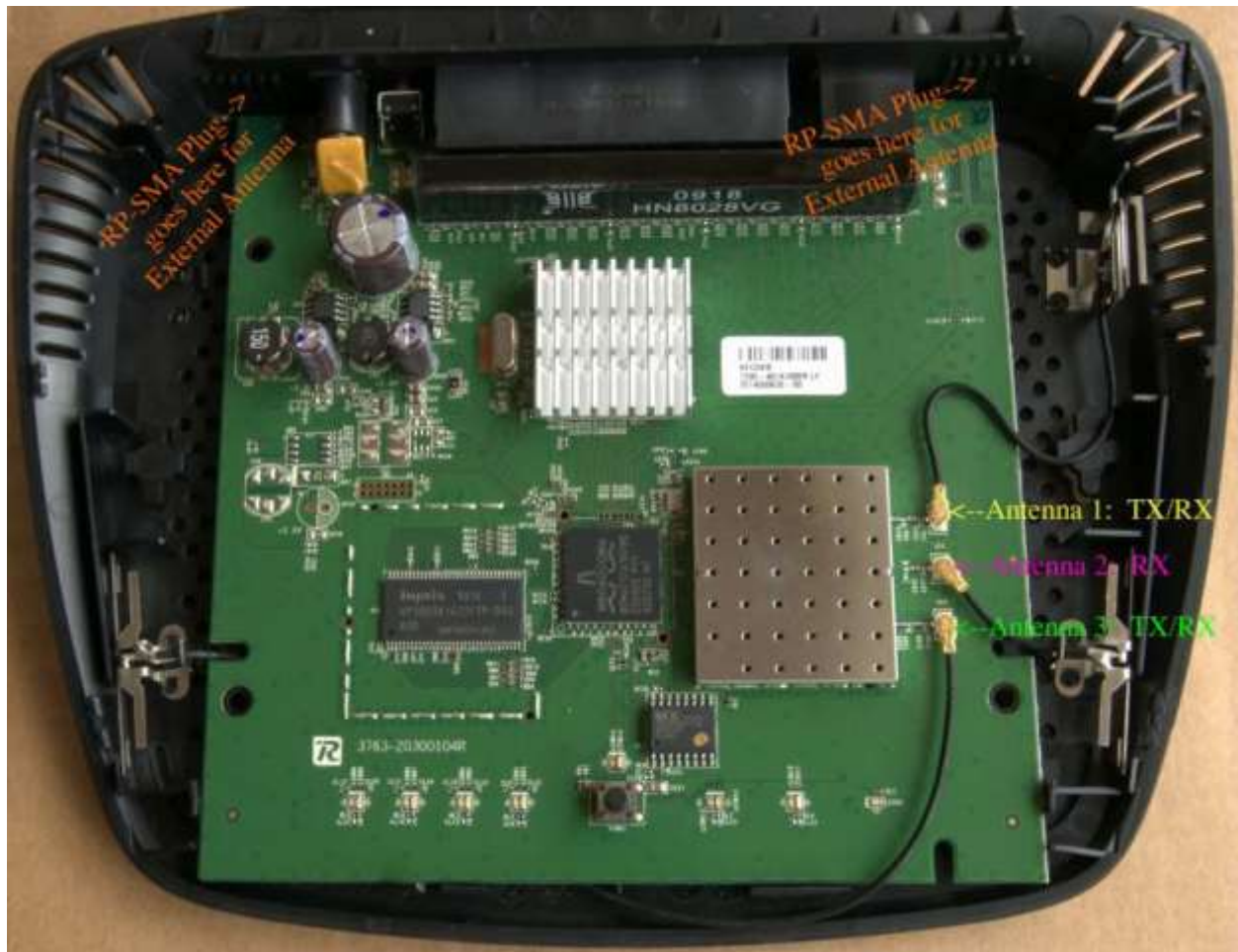
Inside of the E2000/WRT320N: Before the antenna modification
