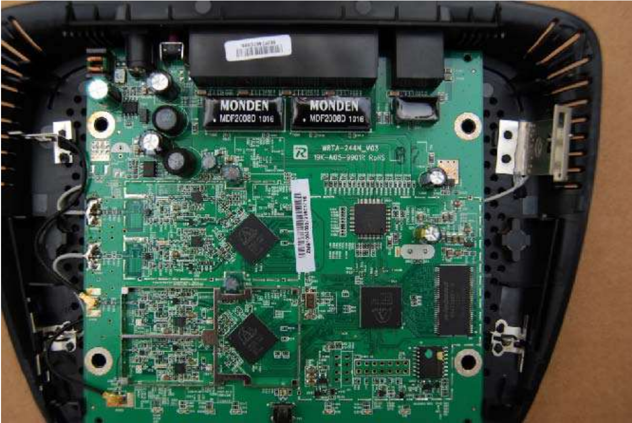
Inside of the WRT400N: Before the antenna modification
