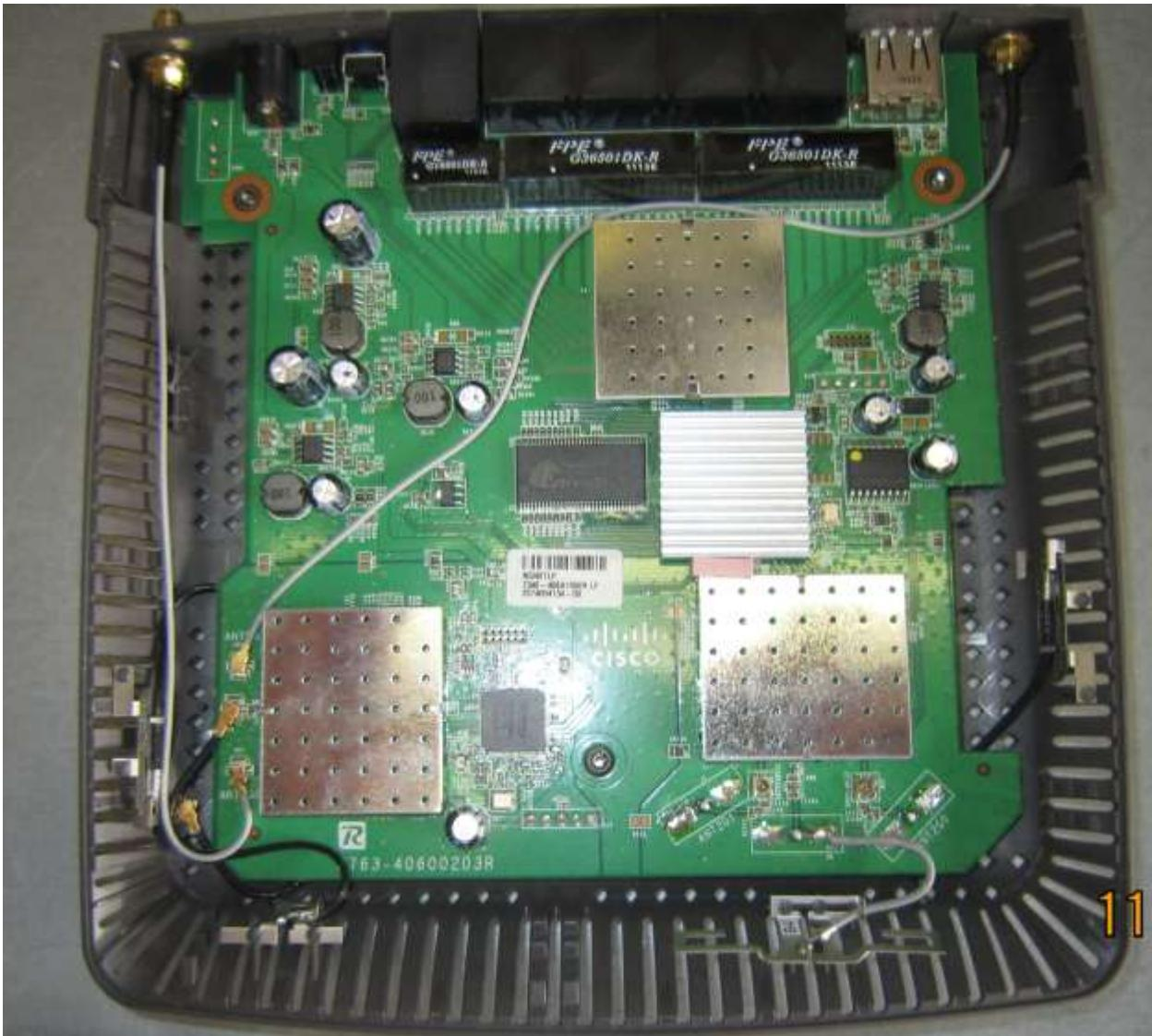
NOTE: When putting the case back together make sure none of the cables get pinched with screws or case. You can secure them in place by using clear tape.
