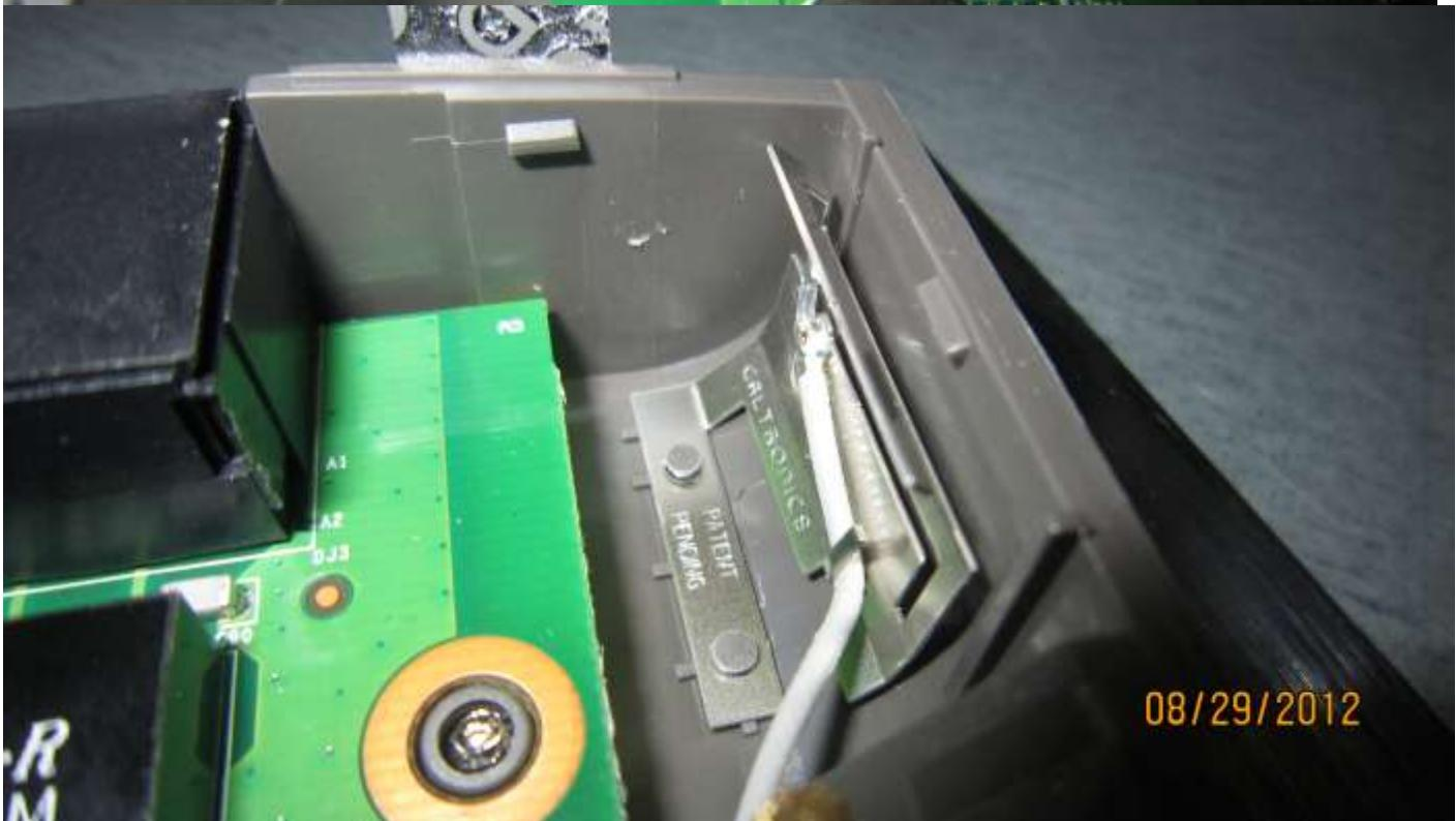
11. Your mark should be just a fraction above center point so the RP-SMA adapter will clear the board.
