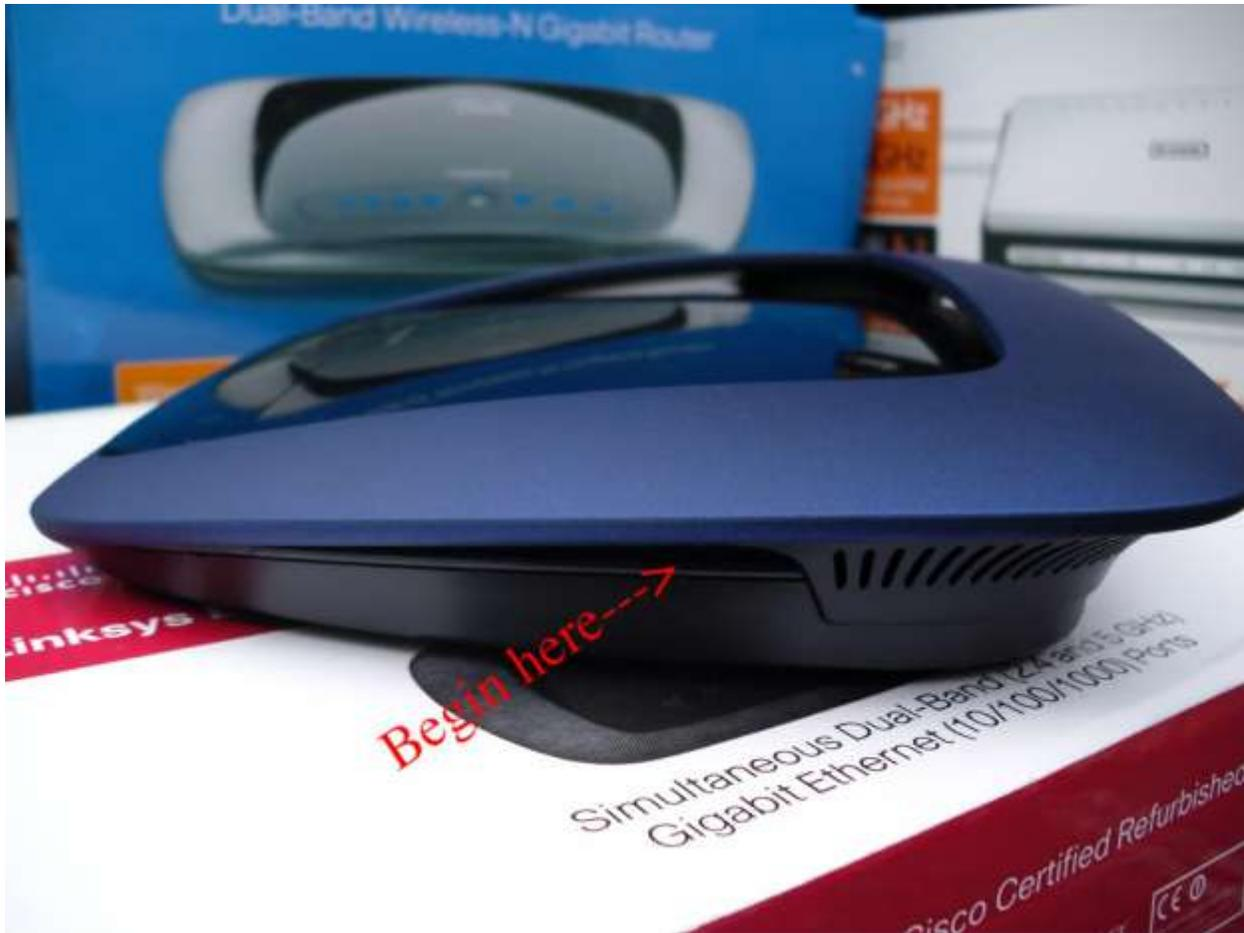
**The top and bottom of the router separate nicely with some help from you.**
