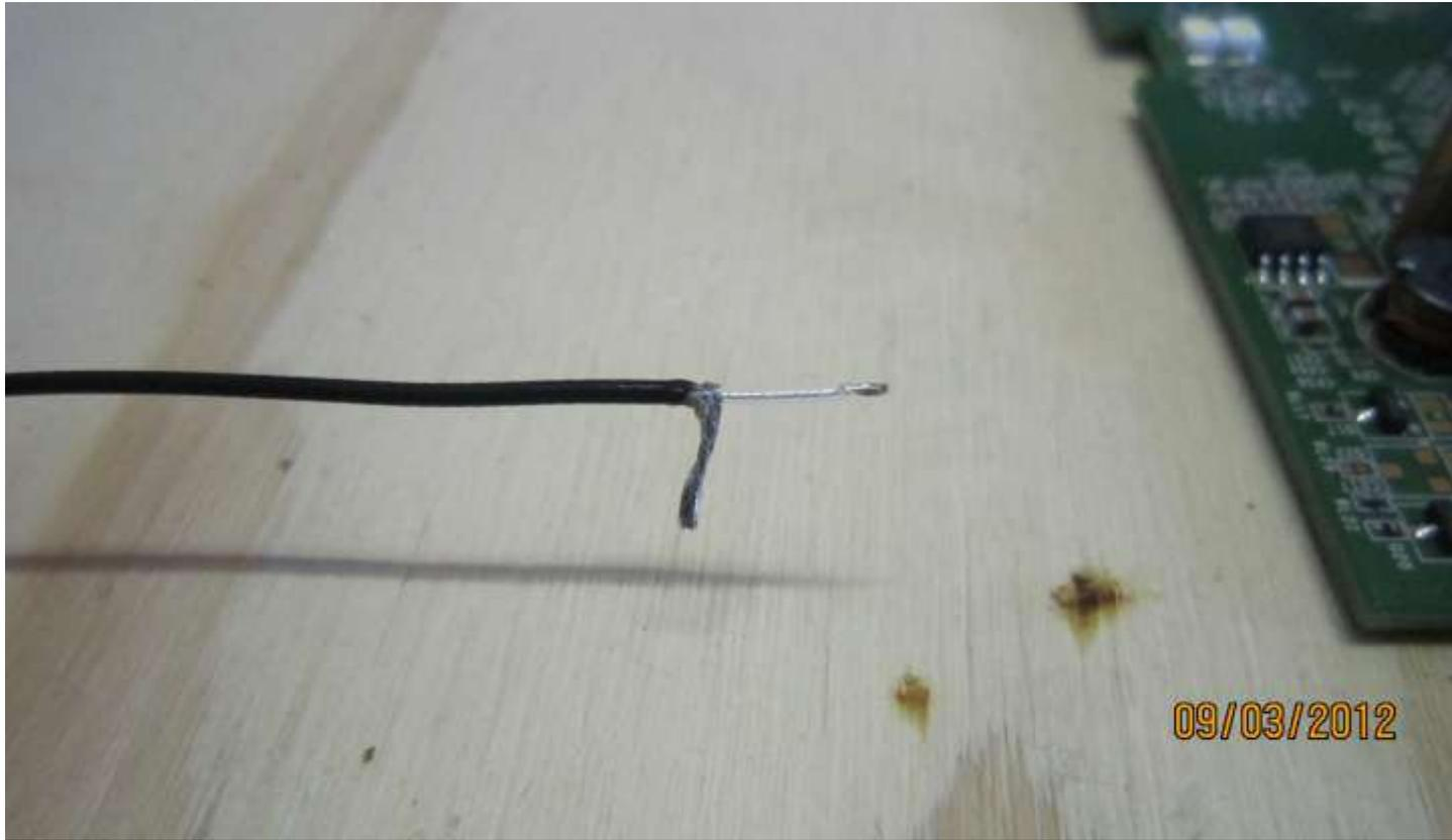
Use a needle to separate the outer portion of cable see below:
