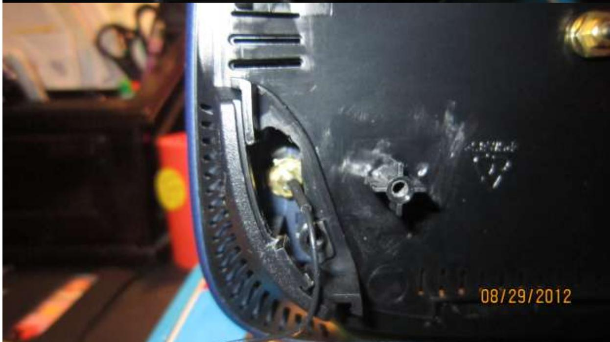
The placement of the 2 center holes doesn't have to be exact but make sure to use picture bellow for reference to avoid hitting some components.
