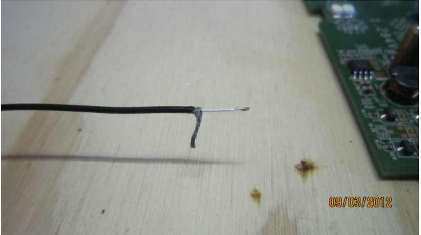
Use a needle to separate the outer portion of cable see below:
