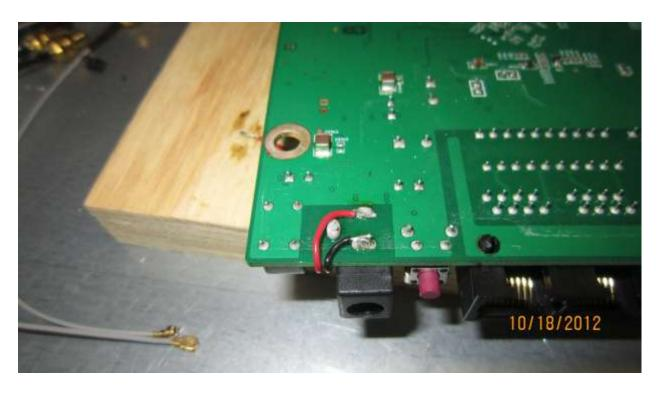
Next step is drilling holes for the fan mount screws. Use 7/64 inch drill bit (or closes you can get to that) Or you can do 5/16 holes like this: (e3000 shown)
