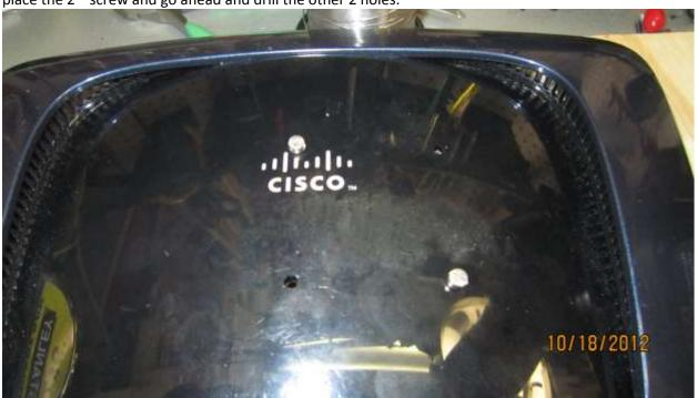
Once 4 holes are drilled you can mark the fan location with a pencil.
