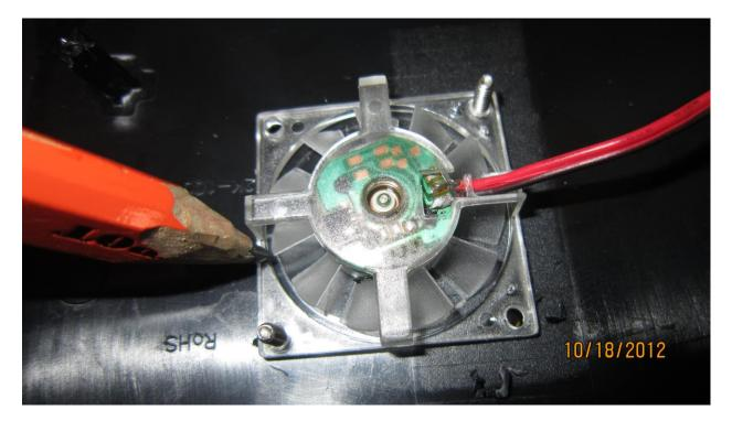
Remove the screws and draw the target using a sharp pencil or a pick. Make sure you do it from the inside of the case.
