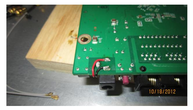
Next step is drilling holes for the fan mount screws. Use 7/64 inch drill bit (or closes you can get to that)
