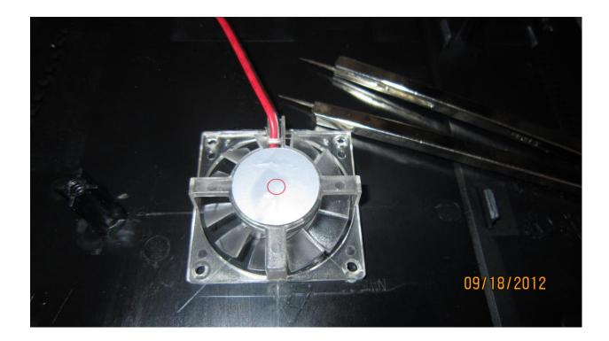
Once 4 holes are drilled you can mark the fan location with a pencil.
