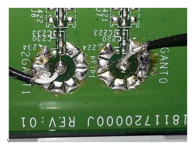
Take your time and make sure each solder is done properly, use the volt meter on each end of the wire to test the contact.
