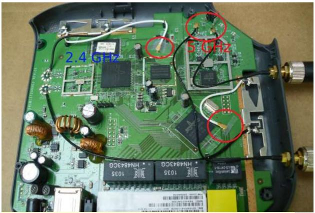
Two external antennas attached to the 5 GHz Frequency Band (no soldering). Notice we have detached the two u.fl internal antenna connectors and taped them to the board.
