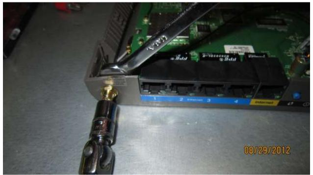
Be sure the nut on the RP-SMA plug is nice and tight (use 8mm wrench and socket here), otherwise your antennas will flop.
