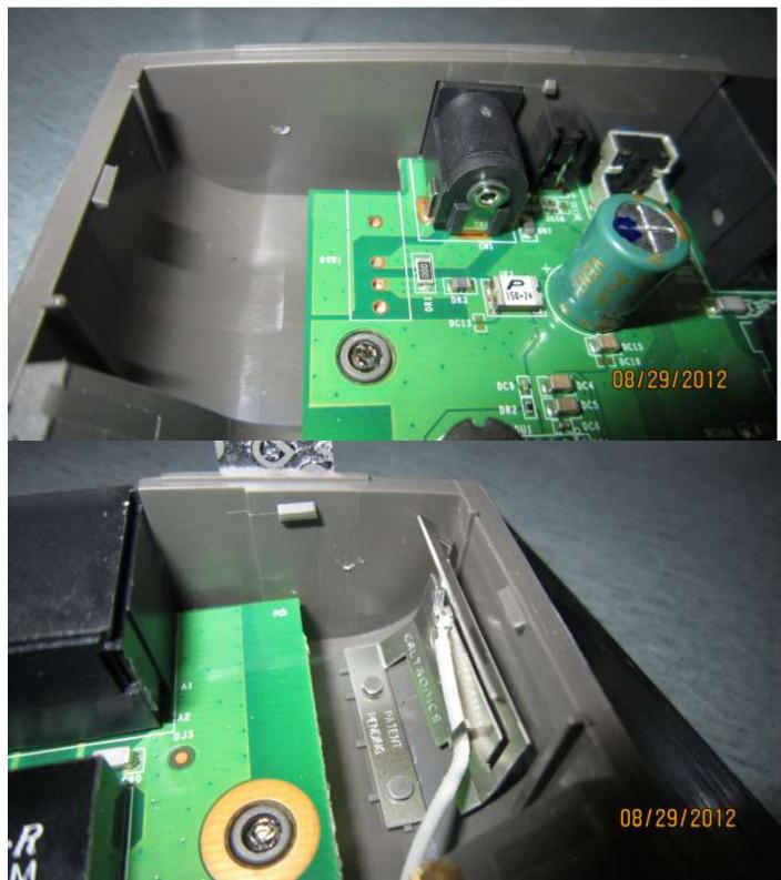
Your mark should be just a fraction above center point so the RP-SMA adapter will clear the board.
