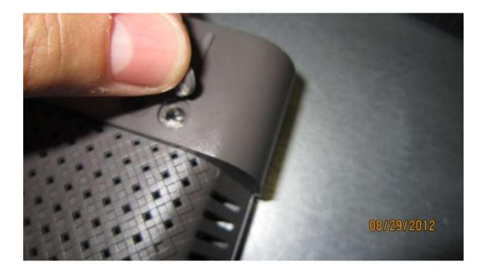
The top and bottom of the router separate nicely with some help from you. Wedge them apart with a kitchen knife or an object that is not sharp. Begin prying the unit open just down from the vent holes. The case is on tight, so pry open around the edges a little at a time. Be patient; she'll eventually pop open for you. If you brake couple of clips don't worry about it, happens to the best of us.
