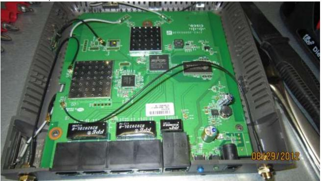
NOTE: When putting the case back together make sure none of the cables get pinched with screws or case. You can secure them in place by using clear tape. Enjoy
