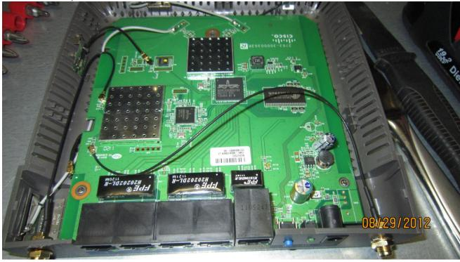
NOTE: When putting the case back together make sure none of the cables get pinched with screws or case. You can secure them in place by using clear tape.
