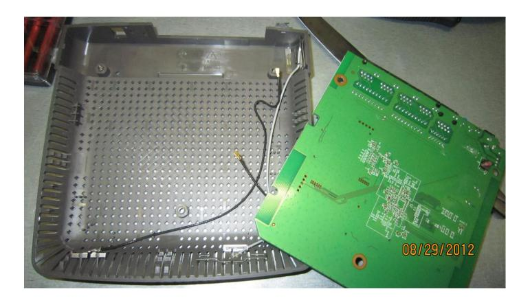
10. Mark on the unit with a pen or whatever you want to use, where you want to drill (see image bellow where the antenna is mounted). Make sure measure it with main board in place to see how much space you need to clear it. If you drill too low you won't be able to insert the U.Fl cables!
