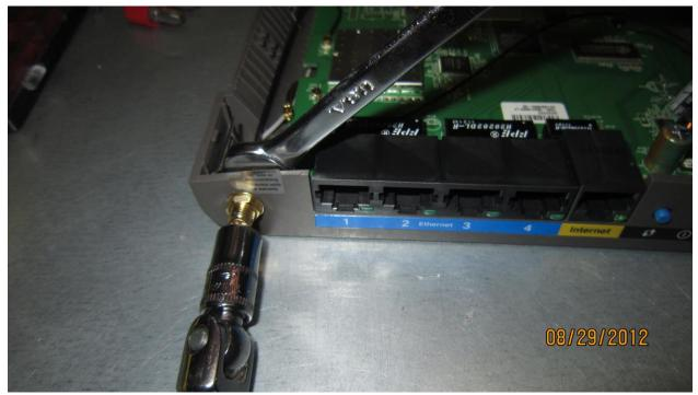
Be sure the nut on the RP-SMA plug is nice and tight (use 8mm wrench and socket here), otherwise your antennas will flop.
