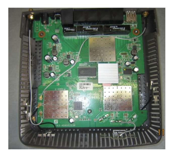
NOTE: When putting the case back together make sure none of the cables get pinched with screws or case. You can secure them in place by using clear tape. Enjoy
