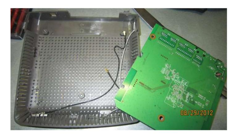
10. Mark on the unit with a pen or whatever you want to use, where you want to drill (see image bellow where the antenna is mounted). Make sure measure it with main board in place to see how much space you need to clear it. If you drill too low you won't be able to insert the U.Fl cables!
