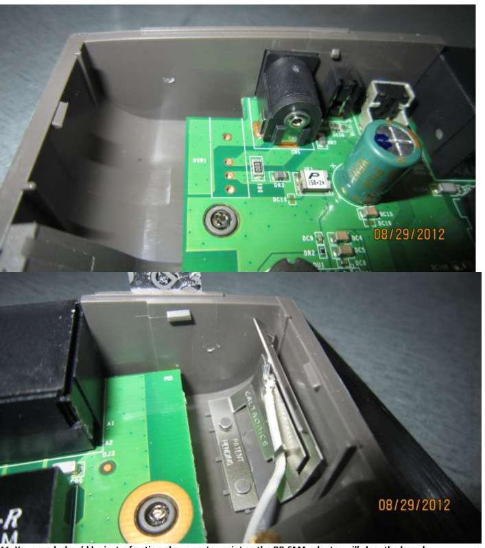
11. Your mark should be just a fraction above center point so the RP-SMA adapter will clear the board.
