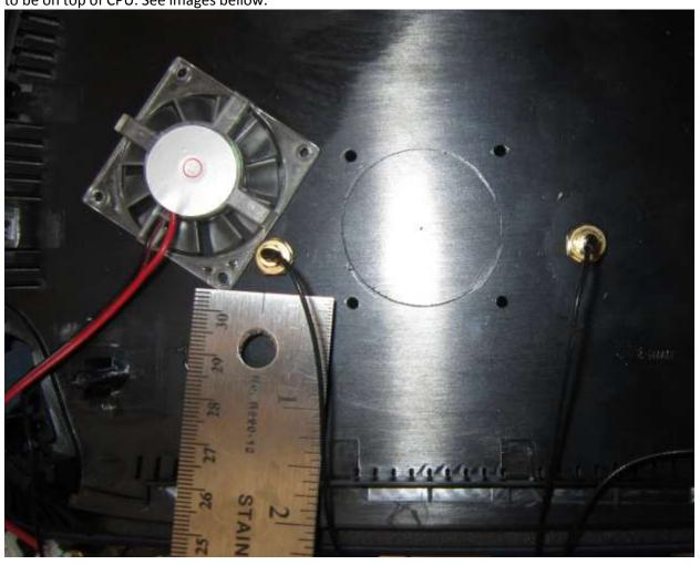
As you can see the hole should be on the side of the Cisco logo. Once you drill the first hole place the fan and secure it with one screw and level it. Now drill the 2<sup>nd</sup> hole through the fan pre drilled hole. Now place the 2<sup>nd</sup> screw and go ahead and drill the other 2 holes.
