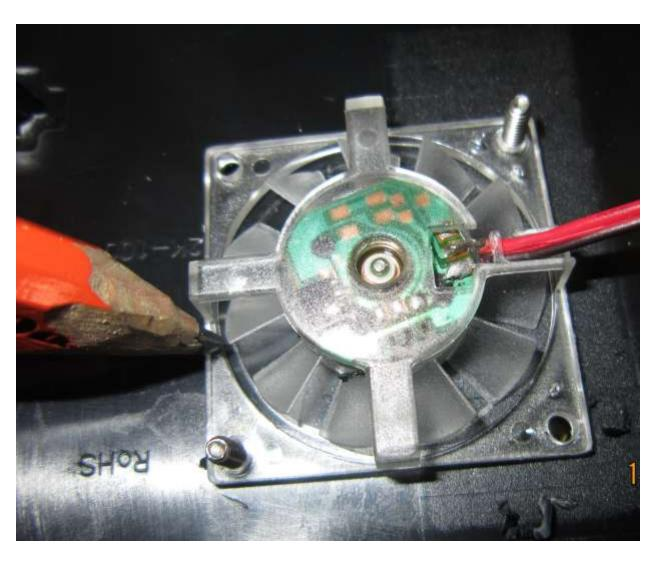
Remove the screws and draw the target using a sharp pencil or a pick. Make sure you do it from the inside of the case.
