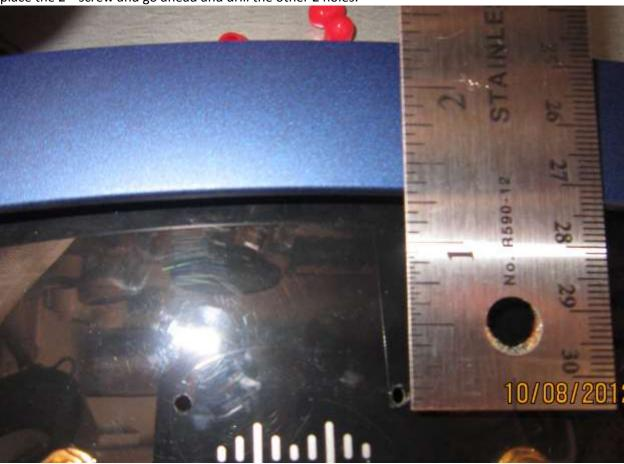
Once 4 holes are drilled you can mark the fan location with a pencil.
