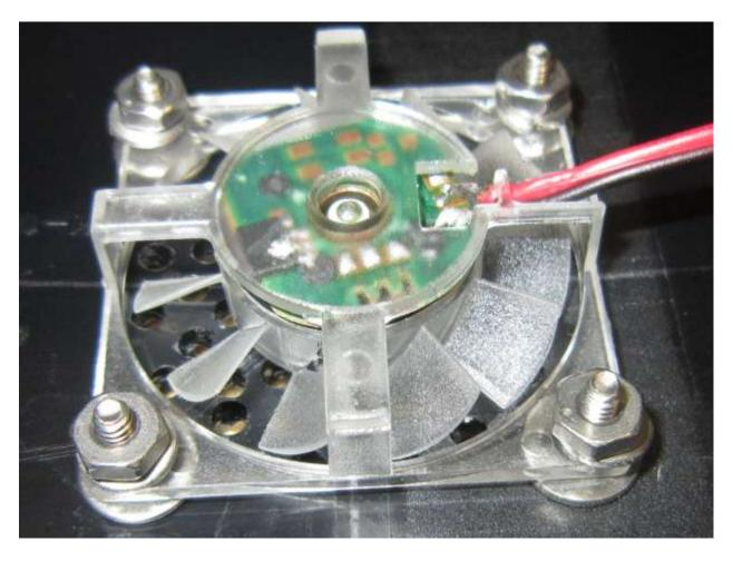
Tighten the screws from the top using flat screw driver. The lock washers will hold the nut in place.
