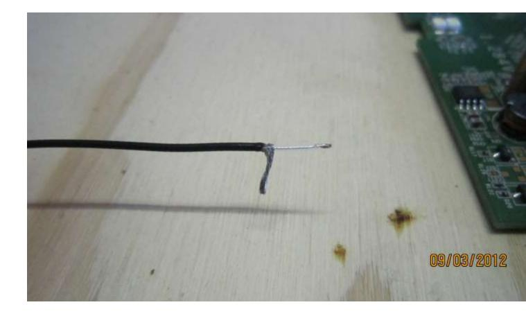
Use a needle to separate the outer portion of cable see below:
