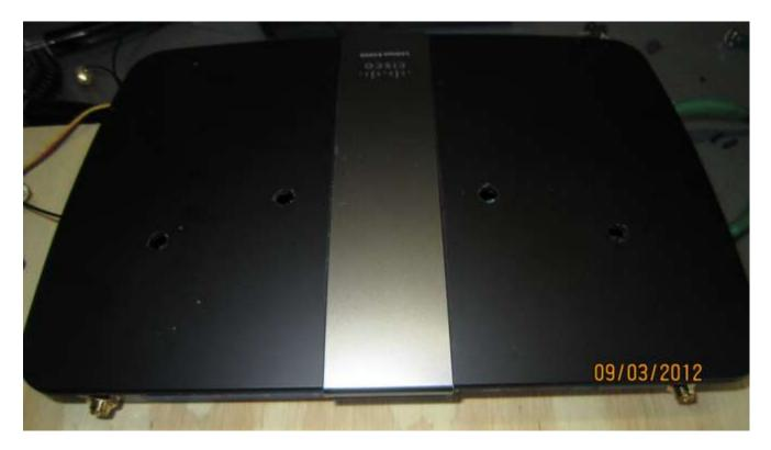
14. After drilling there will be a little plastic left around the inside hole that will need removing. Just use a kitchen knife or other small knife to remove the plastic.
