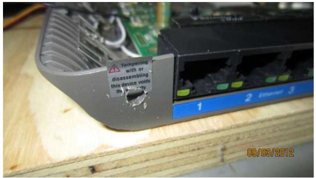
11. Your mark should be just a fraction above center point so the RP-SMA adapter will clear the board. <<Very important IF YOU DRILL TOO LOW THE BOARD WON'T CLEAR
