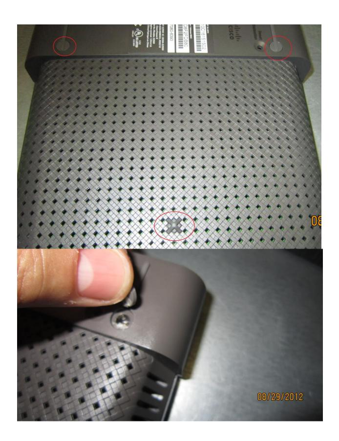
The top and bottom of the router separate nicely with some help from you.
