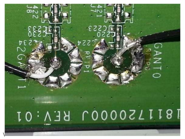
Take your time and make sure each solder is done properly, use the volt meter on each end of the wire to test the contact.
