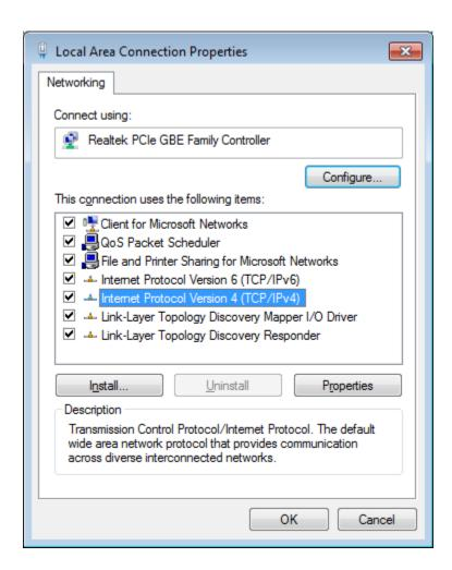
STEP 6: CLICK ON USE FOLOWING IP and INPUT IP, MASK, GATEWAY
