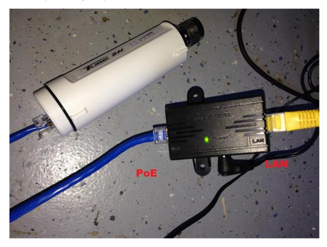
After you configure Tube 2H (must use Static IP), you can now connect to your router (R36 shown here).
