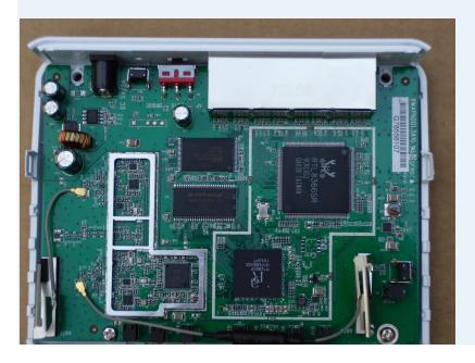
Note: The two internal antennas are called type PIFA ( Planar Inverted F Antenna , antenna planar inverted F)
