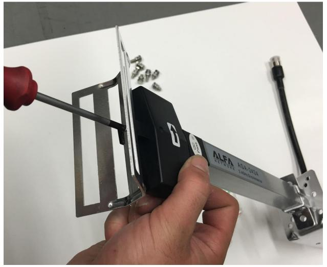
Step 2: Attach 4 screws into Grid of the antenna, please note use shorter screws (longer screws are for middle location, do not install them yet). See how the antenna comes together.
