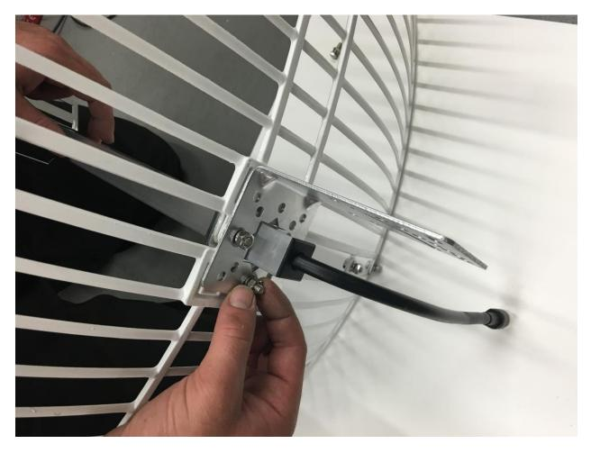
Step 4: Attach the screws through the feed and the L bracket.
